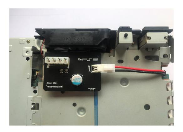
6- Remove the plate with the AC input and the ON/OFF switch by sliding it upwards.
