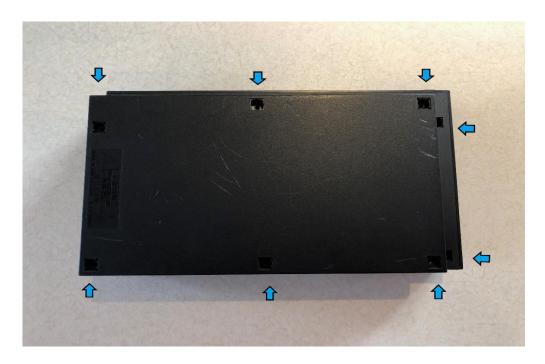
**2- Remove** the top shell and unscrew the two screws holding the controller ports (for some revisions, be careful with the ribbon that connects to the Reset & ON/OFF buttons).
