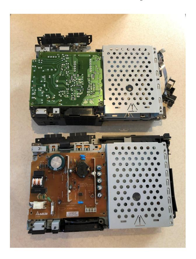
4- Unplug the cable that connects to the ON/OFF switch and pull the PSU upwards (pay attention to the area around the 4-pin connector).
