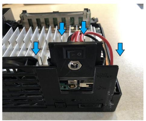
8- Push the small clip that holds the new plate in place.
