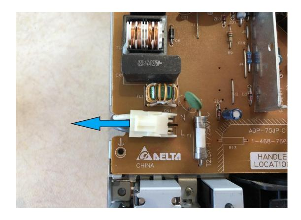
5- Now you can plug the RePS2 PCB on the 4-pin connector and route the cables through the notch that leads to the other side of the board.
