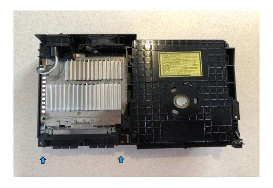
**3- Remove** the bottom shell of your console and flip the whole console over. You should be able to have access to the stock PSU now. Your console should look like one of the two below. Unscrew the 4 screws holding the stock PSU.
