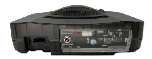
**3**- Finally, plug in a 12v 5A 5.5\*2.1 positive centre adapter. Since the DC jack of the **Re64** is deeper in order to have enough length when installing the 3d-printed bracket, I advise getting a barrel that is 11-12mm in length. Enjoy!
