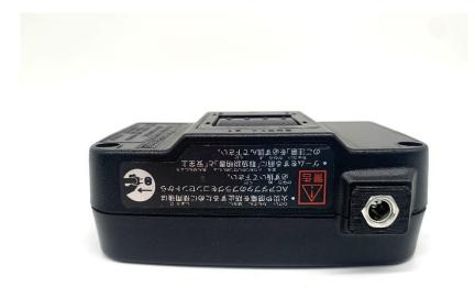
If your shell has the smaller opening, you won't need the 3d bracket, and you can just use the nut to tighten the DC jack into the shell's wall.
