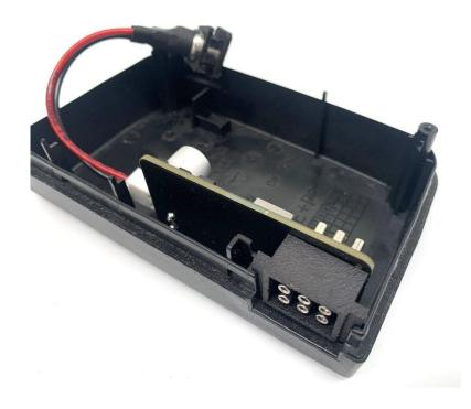
**3-** In order to be able to close the shell properly, you will need to check the opening that your PSU has for the DC jack. As you can see in the pictures below, there is one type of shell with a larger opening than the other:
