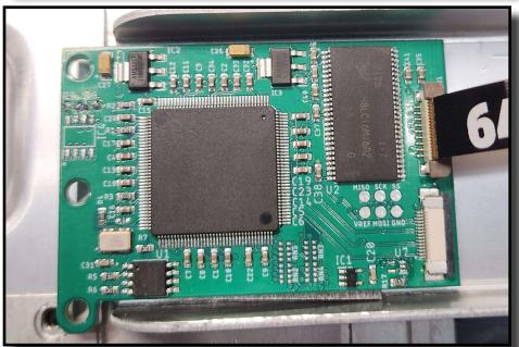
Replace the N64 motherboard. Install the no-cut A/V shroud. Install the top motherboard shield. Remove the screws shown, line up the 64HD main PCB, and reattach the screws.
