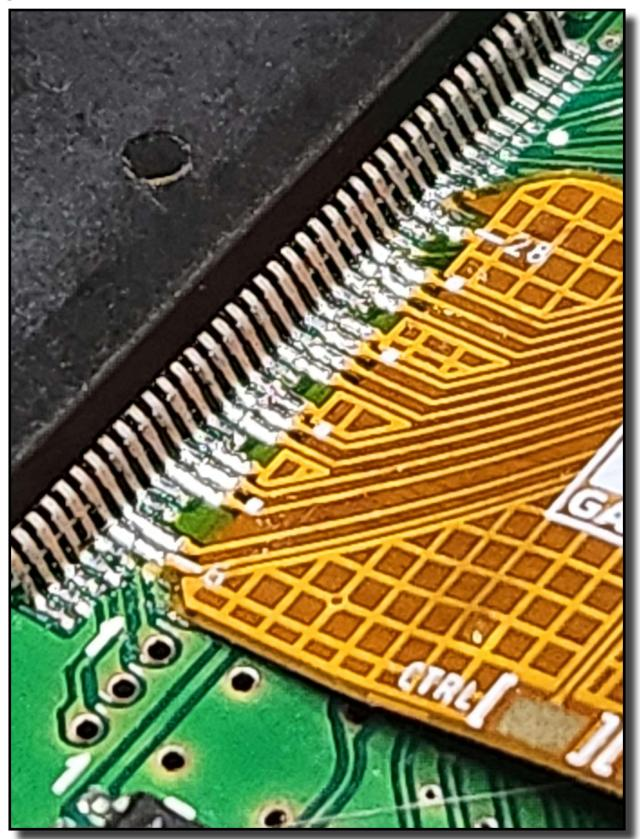
Solder the RCP flex cable starting at Pin 6 (as shown above). Use leaded solder and lots of flux. This is very technical soldering, and mistakes can either ruin your cable, or damage the chip itself. If you damage your RCP flex cable another can be ordered from the retailer you purchased your kit from.
