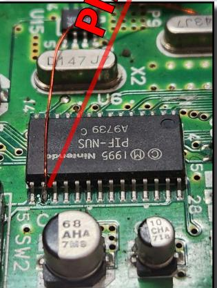
Solder the flex contact to the N64 motherboard location marked "5v" in silkscreen (shown above).
